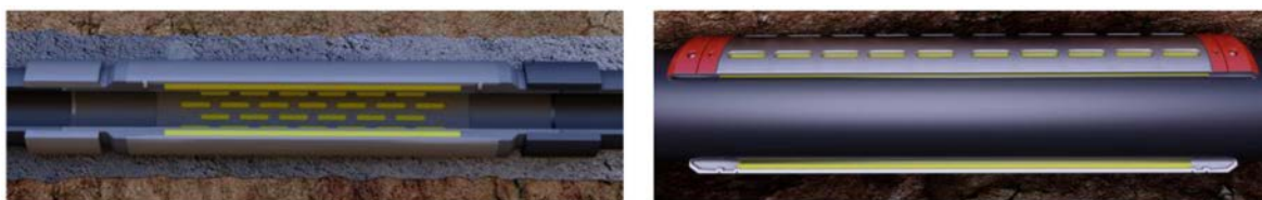
Figure 7—Cross-section view of the tracer sleeves (a) and tracer inserts (b)
