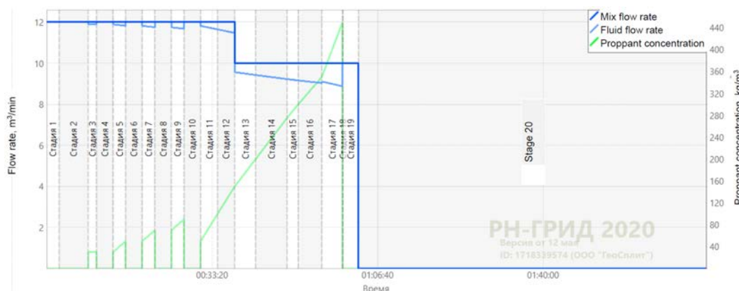
Figure 3—Hydraulic fracturing treatment plan for stages 2-4
