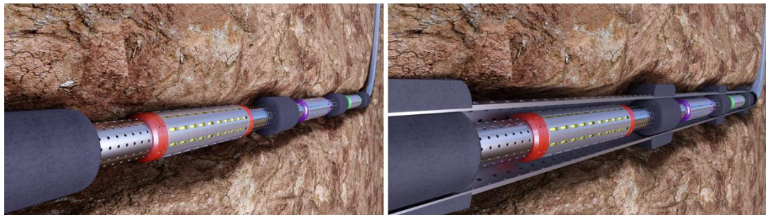
Figure 6 — Placement of marker systems in the lower completion (a) and recompletion (b)
