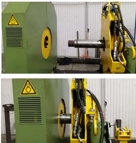
Figure 6—The process of marker cassette prototype model testing on a stand with hydraulic tongs.
