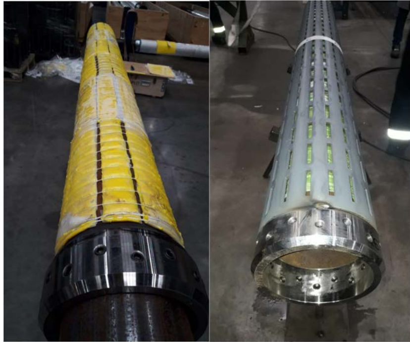
Figure 3—Cassette carrying 3D polymer with markers.
