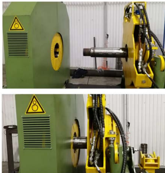
Figure 3—The process of marker cassette prototype model testing on a stand with hydraulic tongs.
